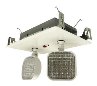
The EL-R2HLED is an energy efficient Emergency Light with two 6V 5.4 watts lamps. Includes maintenance-free backup battery, works on either 120 or 227 VAC.
